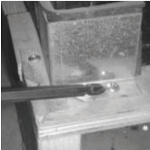
Image 1: Removing bracket from skid
