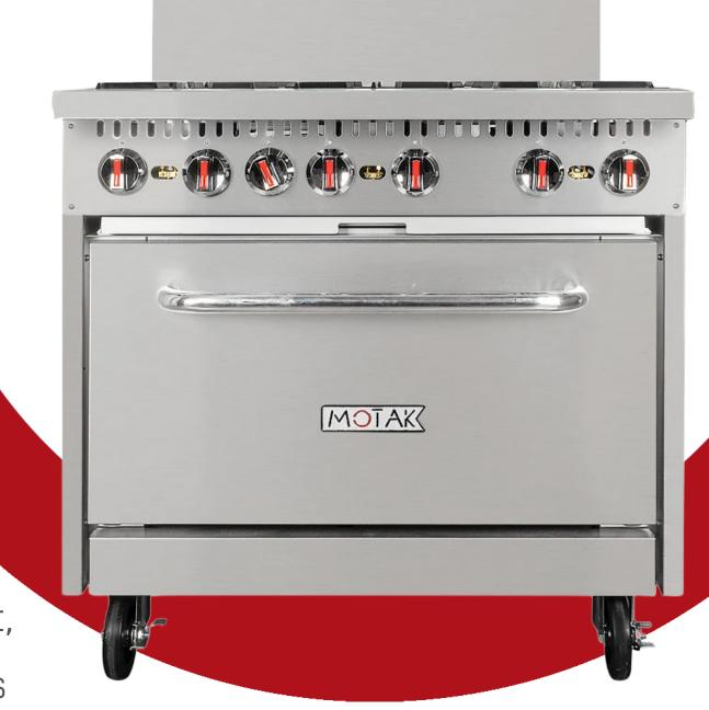
The standard oven has a 30,000-BTU burner, two easy-to-remove oven racks, a porcelain liner for easy cleaning, and a compression spring door hinge system for durability. The oven thermostat adjusts from 200-450°F and is equipped with a flame-failure safety device.
