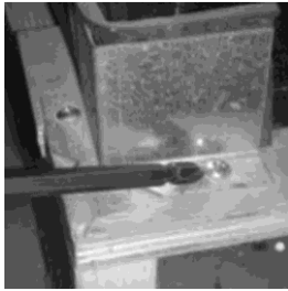
Image 1 Removing bracket from skid
