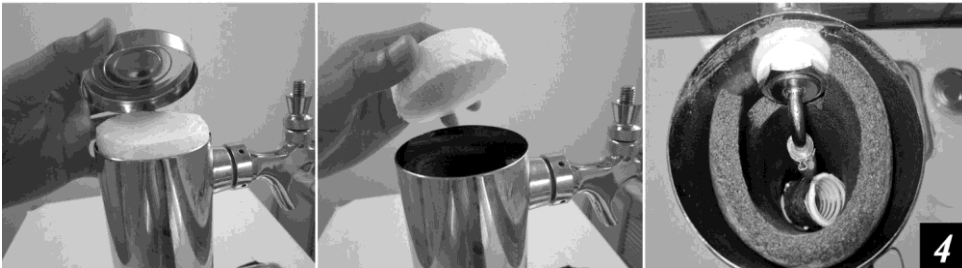
4. Make sure the air hose is always closed at the top of beer tower in order, to keep the beer faucet cold.
