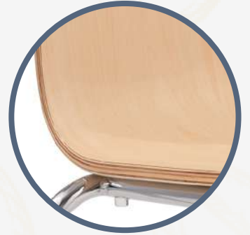
1/2" Thick 8-Layer Bent Plywood Seat With HPL Finish
