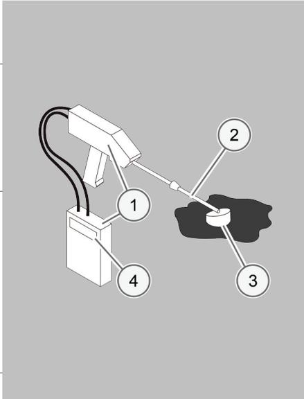
Thread the flue gas analyzer's (1) probe (2) into the exhaust outlet (3) for the burner for which you will be performing the measurement.
