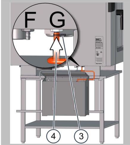
Slip the red suction tube (4) for ConvoClean forte or ConvoClean new cleaning agent onto the barbed nipple on the front bulkhead fitting (G) and secure the tube using the wire hose clamp (3) (see 'Cleaning-agent connection' adhesive label on the left unit side).
