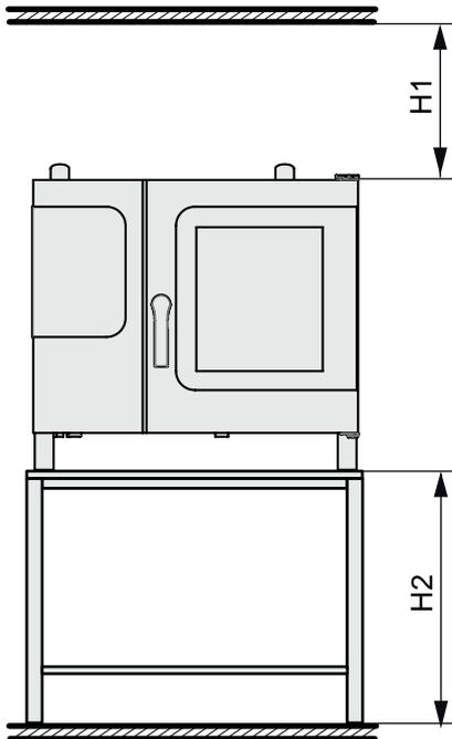
The service technician responsible for setting up the unit must take into account the ceiling's properties and any adjacent systems being used (air ventilation system, range hood) when determining the actual clearance required between the top of the unit and the ceiling. Vertical clearance H1 is only meant to serve as a reference point for the minimum vertical clearance.
