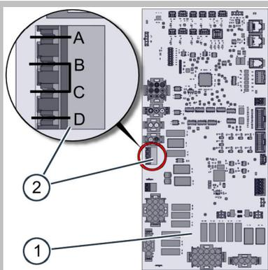
Remove the jumper between terminals (B) and (C) on terminal block -X37 (2).
