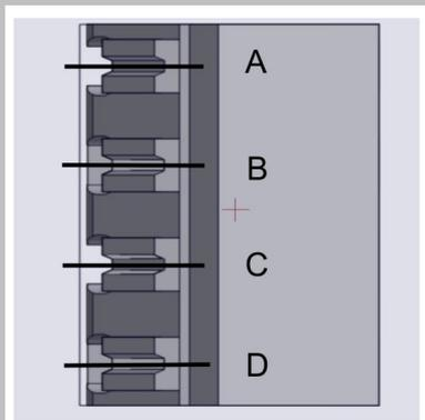
Connect terminals (A), (B), (C), and (D) on terminal block -X37 (2) to the energy optimization system.
