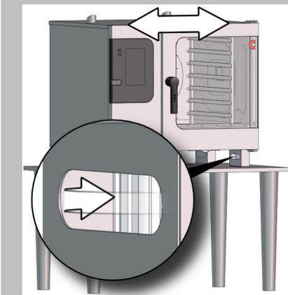
Use the adjusting screw to level the unit. To turn the adjusting screw, use the unit foot tool or water pump pliers. In addition, use a spirit level to make sure that the unit is properly leveled.
