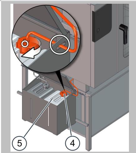
Insert the suction nozzle on the red suction tube (4) into the cleaning agent canister (5). The tube must be routed without any kinks and the canister's vent opening must be open and clear.
