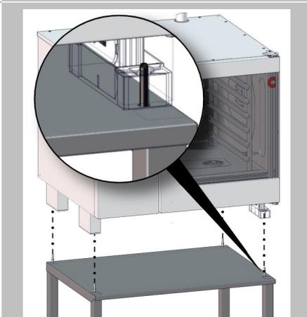
Place the unit on the stand. Make sure that all four studs go into the locating holes at the bottom of the unit's feet.
