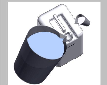
1. Mix the included ConvoCare K concentrate with soft water in the empty canister for ConvoCare rinse aid. Make sure to follow the operating manual instructions on mixing ConvoCare rinse aid in canisters.
