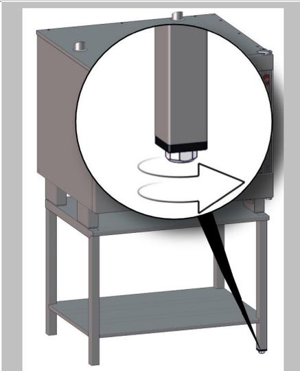
Use the height-adjustable feet to level the stand. Use a spirit level to make sure that the unit is properly leveled. The unit's absolute inclination during operation must not exceed max. 2° (3.5%).
