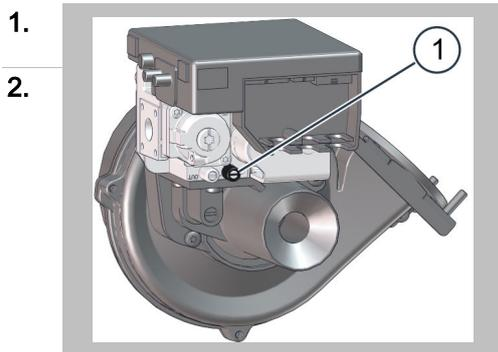
Measure the supply flow pressure at the gas valve (1) on the forced air burner.
