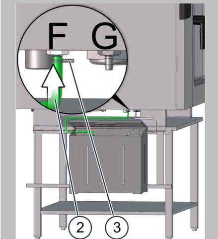
2. Slip the green suction tube (2) for ConvoCare rinse aid onto the barbed nipple on the rear bulkhead fitting (F) and secure the tube using the wire hose clamp (3) (see 'Rinse-aid connection' adhesive label on the left unit side).
