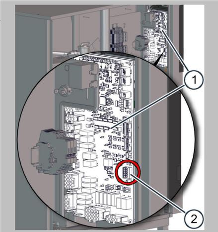
Remove the side panel from the combi oven in order to access terminal block X32 (2) on the system interface board (SIB) (1) in the area behind the operating panel.
