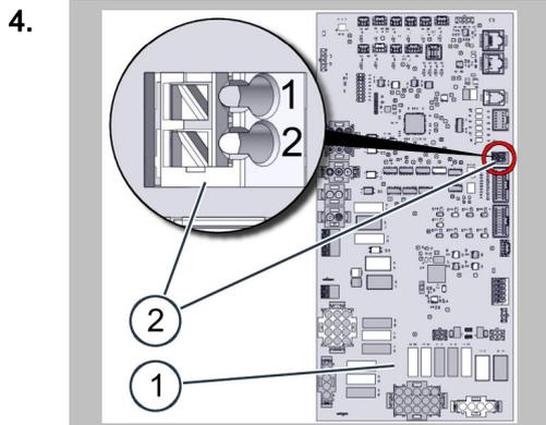
Connect the water treatment filter monitoring system's connection cable to the combi oven, observing the following pinout:
