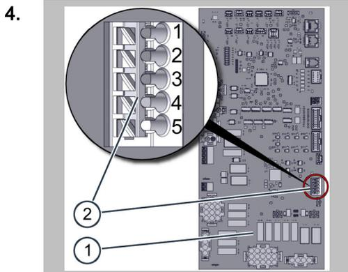
Connect the signal tower's connection cable to the combi oven, observing the following pinout:
