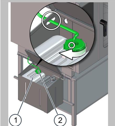
3. Insert the suction nozzle on the green suction tube (2) into the rinse aid canister (1). The tube must be routed without any kinks and the canister's vent opening must be open and clear.
