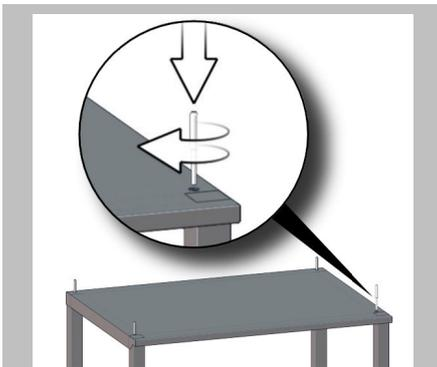
Screw the studs into the corresponding stand threads, then tighten them using the screwdriver.
