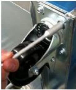
Remove the screws of the casters
