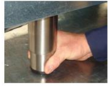
Adjust the legs to level the unit
