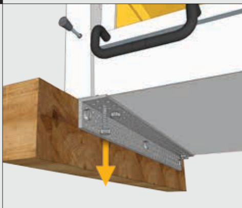
24. Remove the 8 hex bolts M10x30 under the oven and keep them
