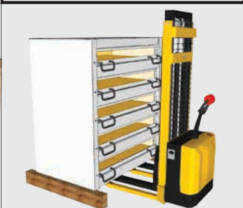
23. Carefully lift the oven using a pallet truck, forklift or Genie lift, depending of the weight of the oven
