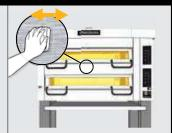
**6. Clean Surfaces**Clean all the stainless steel surfaces with the cloth, always with grain direction.
