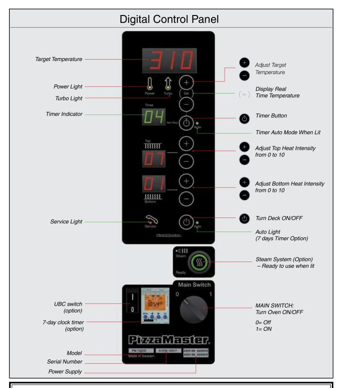
Power: A yellow lamp indicates that the heating element is on.
