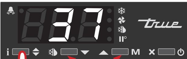
While still holding, press and release the down or up arrow to change the setting.
