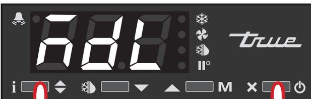
Press and hold until "Mdl" or "SPL" is shown.
