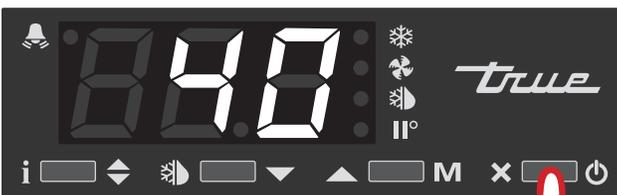
To turn on, press and release until the cabinet temperature is shown.
