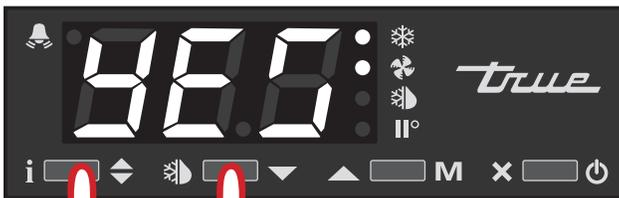
If "Yes", while still holding, press and release down arrow to change to "no" (unlocked).
