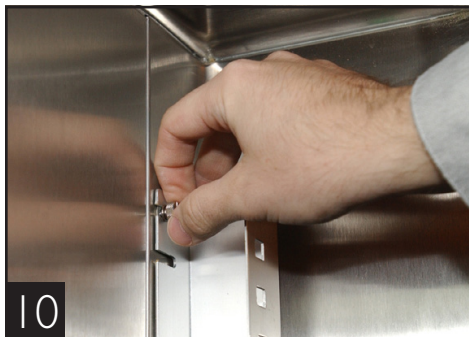
Pilaster installation (side wall of cabinet)
