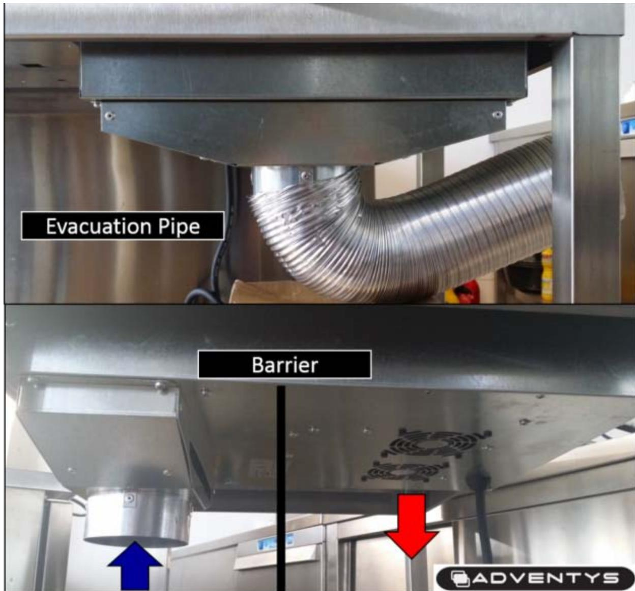
To insure proper ventilation, make sure there is 8" between the bottom of the unit and the surface below. A clearance of 2" is recommended on all sides.
