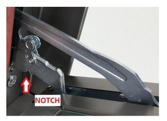
2. Move the hinge lock to the "down" position to restore proper hinge operation
