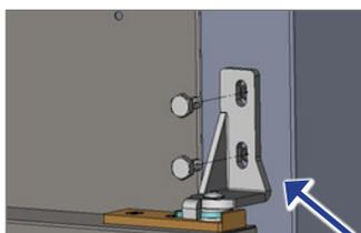
First, ensure the door weight opposite the hinge side is supported. The top hinge bracket bolts can be removed.
