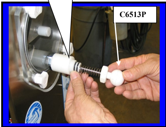
Installing Plunger Assembly into Faucet body
