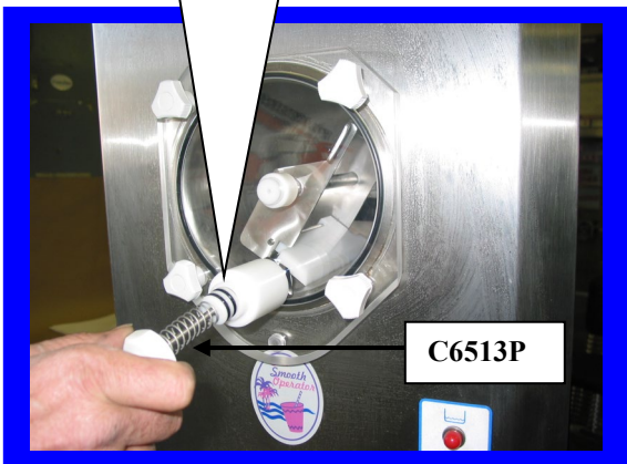
Installing Plunger Assembly into Faucet body
