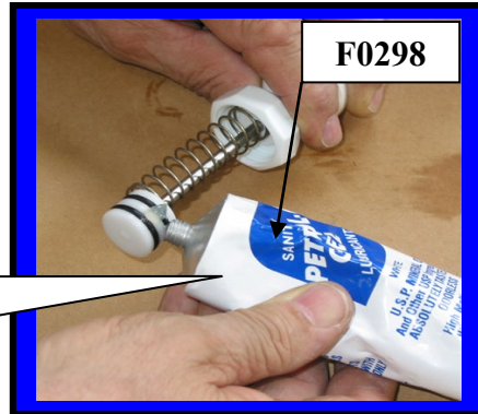
Install O-rings onto plunger
