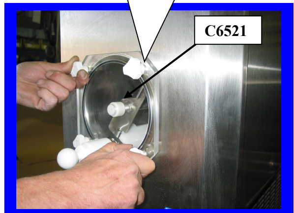
Installing small Faceplate onto front of Machine.
