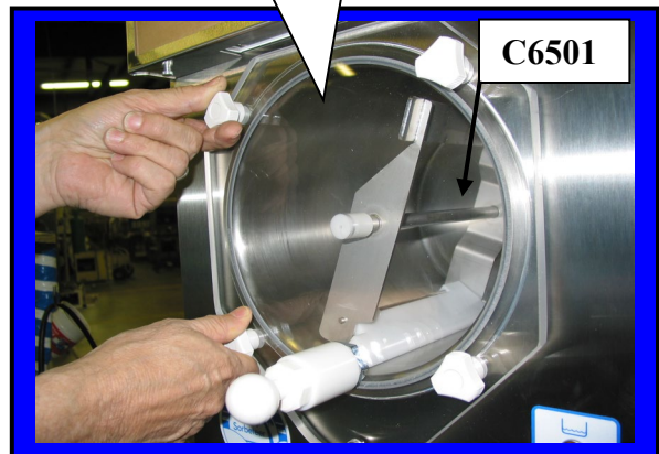
Installing Faceplate onto front of Machine.
