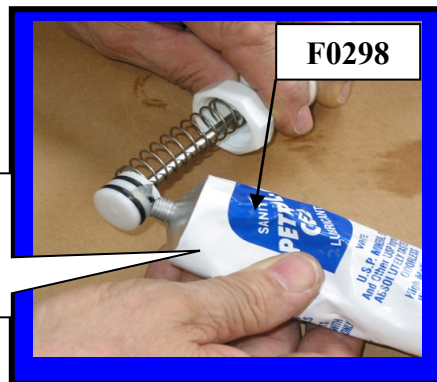
Lubricating O-rings with Petro-Gel
