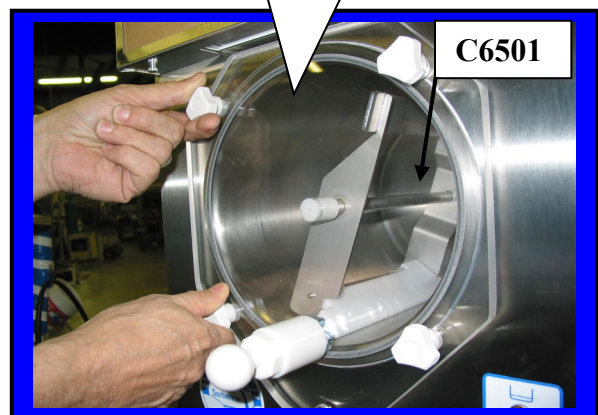
Installing large Faceplate onto front of Machine.
