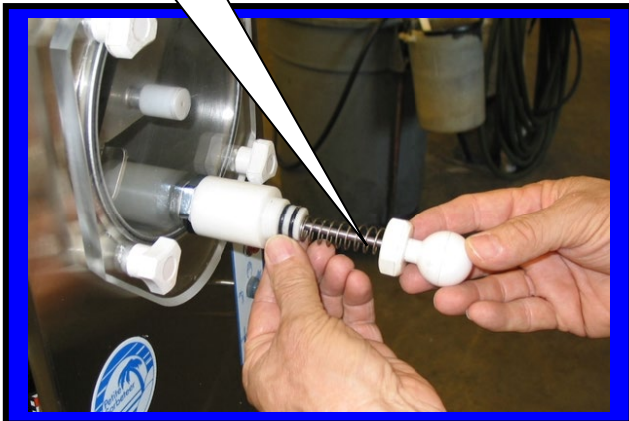
Installing faceplate C6521 onto front of Machine.
