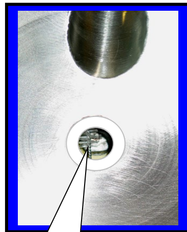
Push brush all the way in until it can be seen in the middle of the ceramic ring
