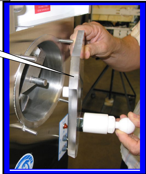
Installing faceplate C6521 onto front of Machine.
