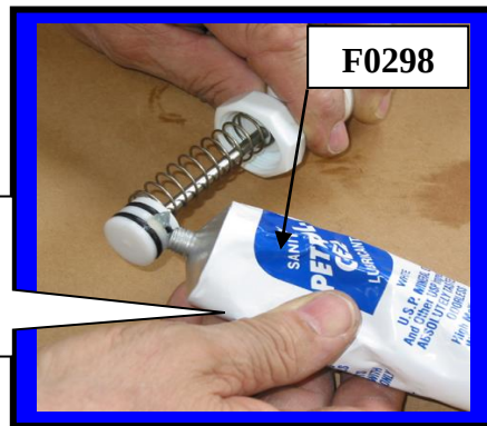
Lubricating O-rings with Petro-Gel
