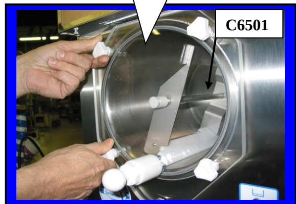
Installing large Faceplate onto front of Machine.
