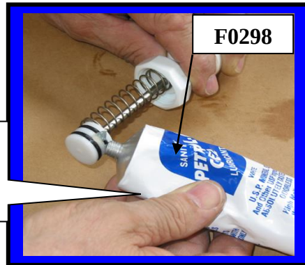
Lubricating O-rings with Petro-Gel
