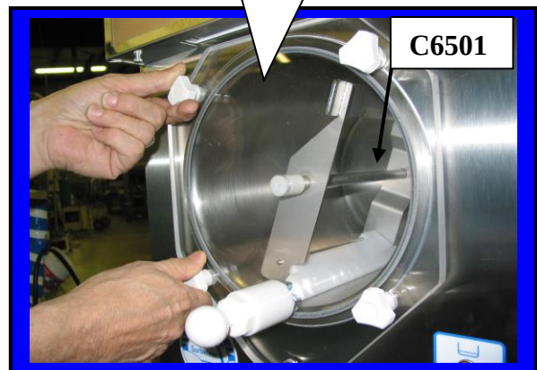
Installing large Faceplate onto front of Machine.
