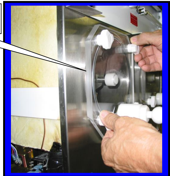
Installing faceplate C6521 onto front of Machine.
