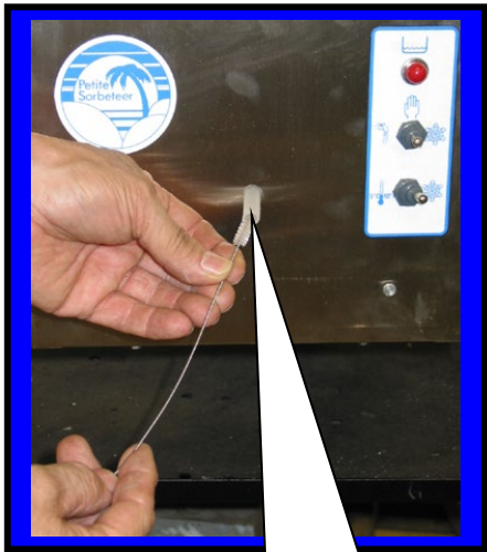
Insert long brush F6526 into drip tube
