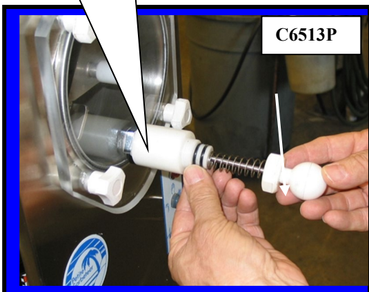
Installing Plunger Assembly into Faucet body
