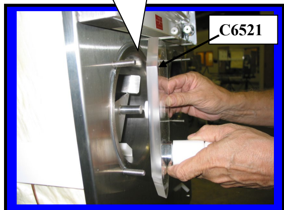
Installing Faceplate onto front of Machine.
