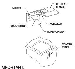
MOUNT APPLIANCE SO THAT THE CONTROL PANEL IS LOCATED TO THE FRONT OF THE FIXTURE.
