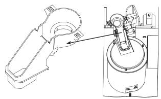
14. The ice chute can be cleaned in place. If complete removal is desired, use a Phillips screwdriver to remove the Hall Effect switch assembly from the ice chute.
