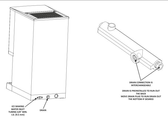
**Typical Water Supply Drain Installation**
