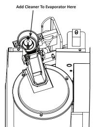
**Step 3** The ice machine will run a wash cycle, a series of rinse cycles and then stop. This entire cycle lasts approximately 30 minutes.
