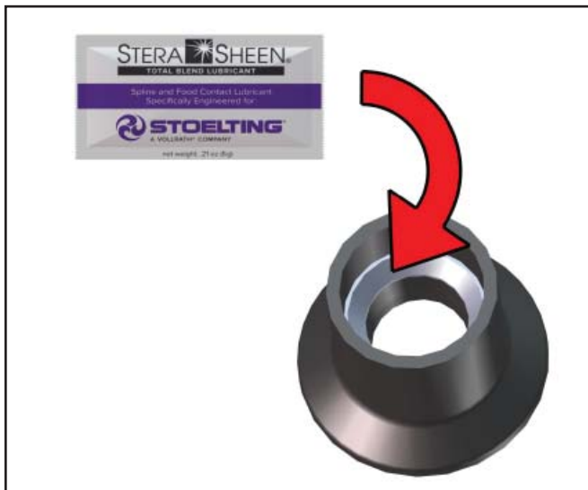
Figure 3-5 Lubricate Rear Seal
