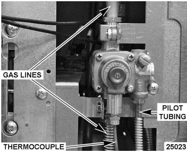
**Gas Safety Valve on 30" Convection Oven**
