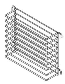
Example shows 9 level rack with 25%" spacing
