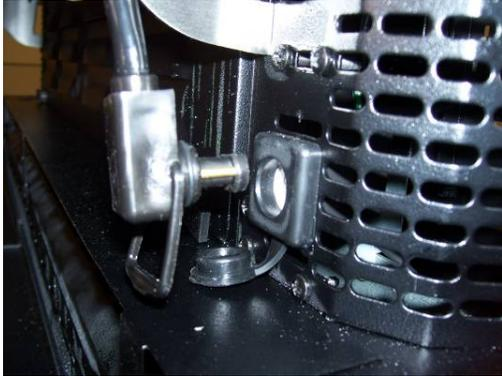
8. Place extra cord into cord clip as shown to keep it out of the way.
