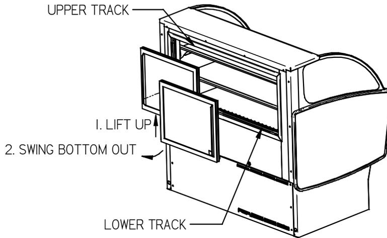
1. Start with the outer door and lift the door upward until the bottom edge of door clears the lower track and then swing the bottom of the door outward and down out of upper track.
