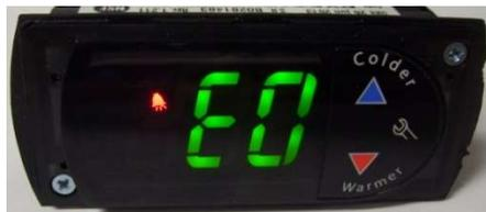
You may mute the alarm by pressing and releasing the wrench button. The red ringing bell and all error codes will still be displayed. When the fault is remedied the control will return to normal operation and will automatically clear the codes from the display.
