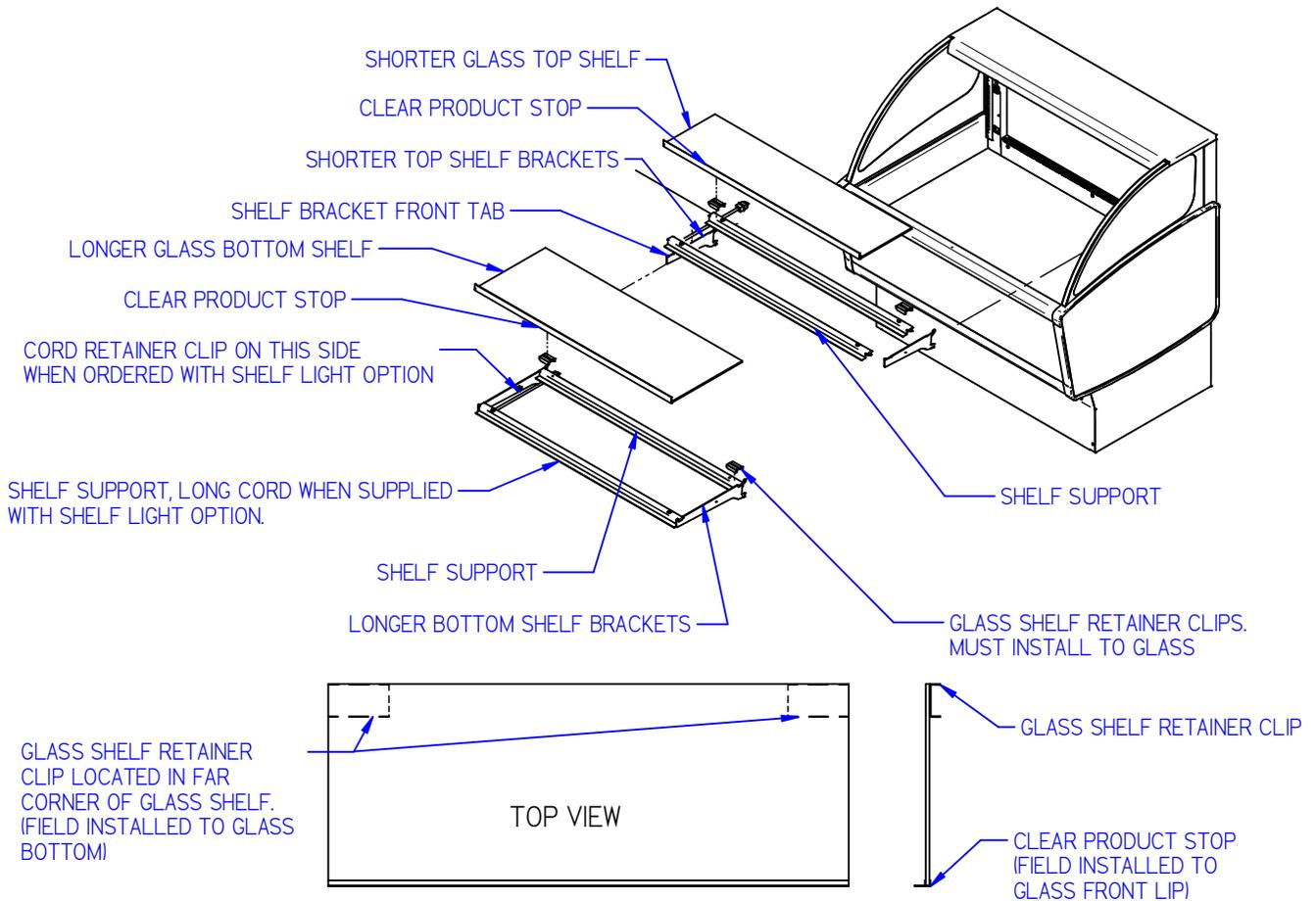
1. When installing for the first time, attach (2) glass shelf retainers to each glass shelf. Remove the backing from the tape located on the flat side of the glass shelf retainer. Position the glass shelf retainer in the (2) far corners of the glass as shown in the above figure. Repeat for each glass shelf.
