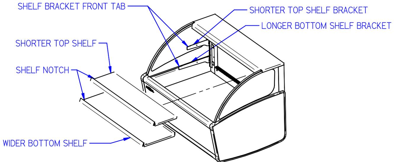
1. Follow the instructions in the illustration below and insert (1) of the shelf brackets in the desired shelf standard slot on one side of the case. Place the additional bracket in the same shelf standard slot on the opposite end of case. If the case was supplied with shelf light option (ELPRSS), the bracket with a clear plastic cord retainer clip must be on the side with the shelf light. For LPRSS case with (2) shelves repeat for shorter top shelf brackets.
