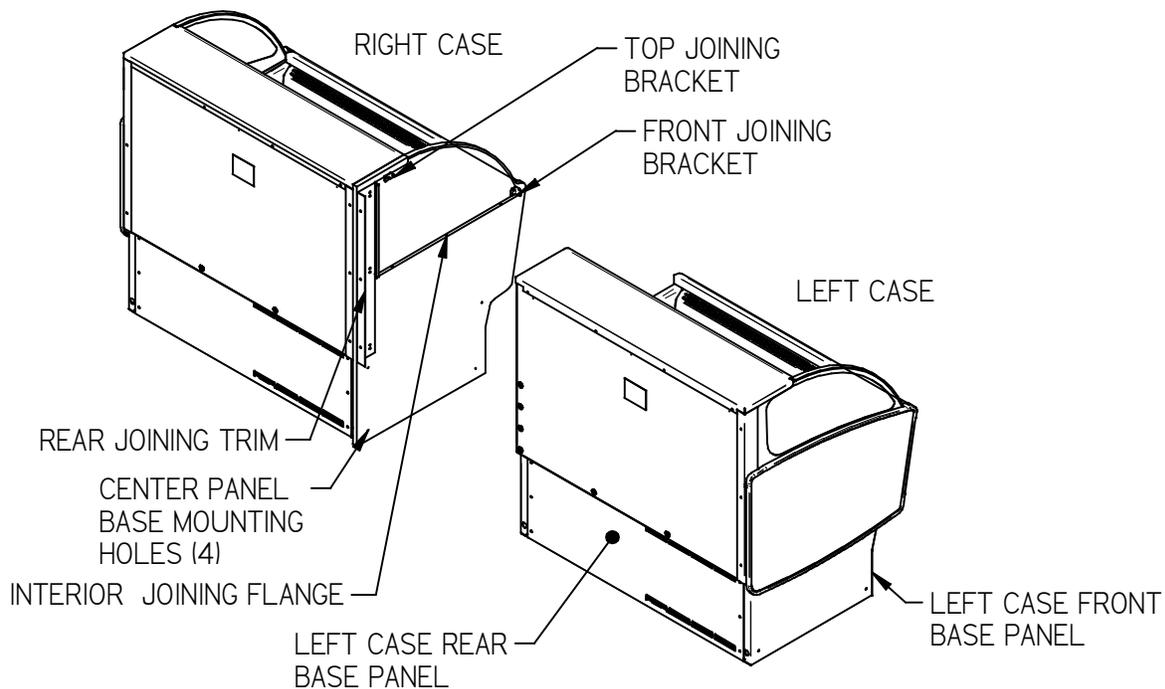
1. Place the right case into desired location and level case by adjusting leg levelers with provided wrench.
