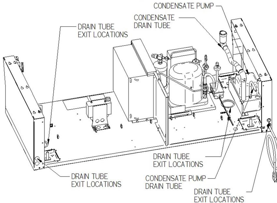
Instead of using heat energy to remove condensate run off from the evaporator coil a condensate pump moves the water to a nearby drain.
