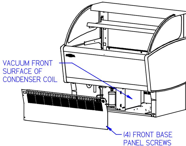
Figure 1 - Condenser Cleaning
