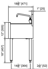
TS (18-9/16"D) & TSF (24"D) Series Three Compartment Sinks (M3) with and without Drainboards
