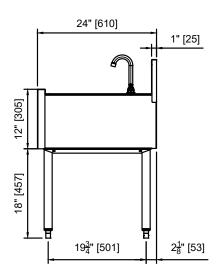
TS (18-9/16"D) & TSF (24"D) Series Three Compartment Sinks (M3) with and without Drainboards
