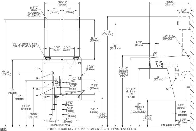
A = Recommended Water Supply location. Shut-off Valve (not furnished) to accept 3/8" O.D. unplated copper tube. Up to 3" (76mm) maximum out from wall. B = Recommended Waste Outlet location. To accommodate 1-1/4" nominal drain. Drain stub 2" (51mm) out from wall.
