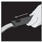
Place fastener (with the dot closest to pan) into the silicone grip-handle hole. Push the fastener down into place with a pointed (not sharp) object.
