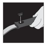
3. Flip the pan over and press around the flange center button to secure the fastener.
