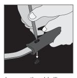
3. Flip pan over and remove the old silicone grip from handle.
