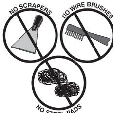
**NOTICE:** Avoid the use of abrasive cleaning compounds, chloride based cleaners, or cleaners containing quaternary salts. Never use hydrochloric acid (muriatic acid) on stainless steel.
