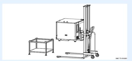
Lower the oven onto the stand. Make sure the legs fit into the pockets on the stand.
