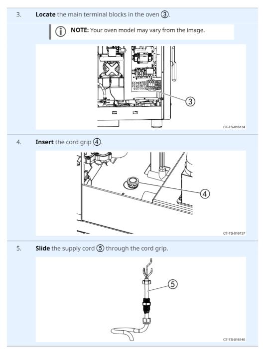
Install the supply cord into the oven far enough to reach the ground terminal block.
