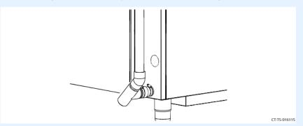
Install the 45° elbow to the Tee. Install the drain pipe. Install the 90° elbow.
