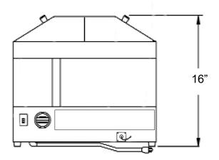
Hot dog compartment dimensions are 6"W x 11"D x 8"H Bun compartment dimensions are 11"W x 11"D x 8"H
