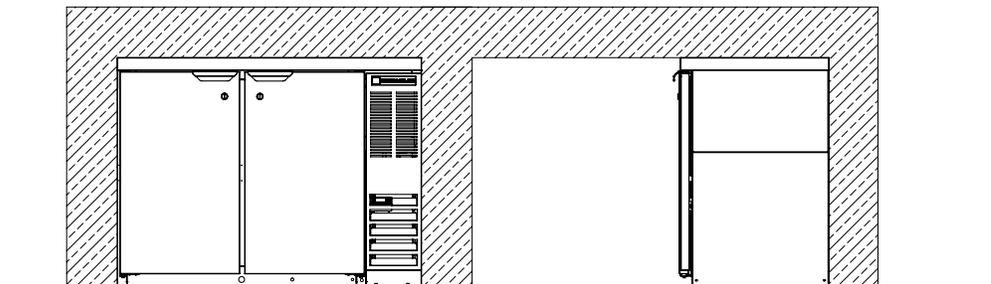
0 INCHES MINIMUM CLEARANCE AT TOP, BOTTOM, SIDES AND BACK.
