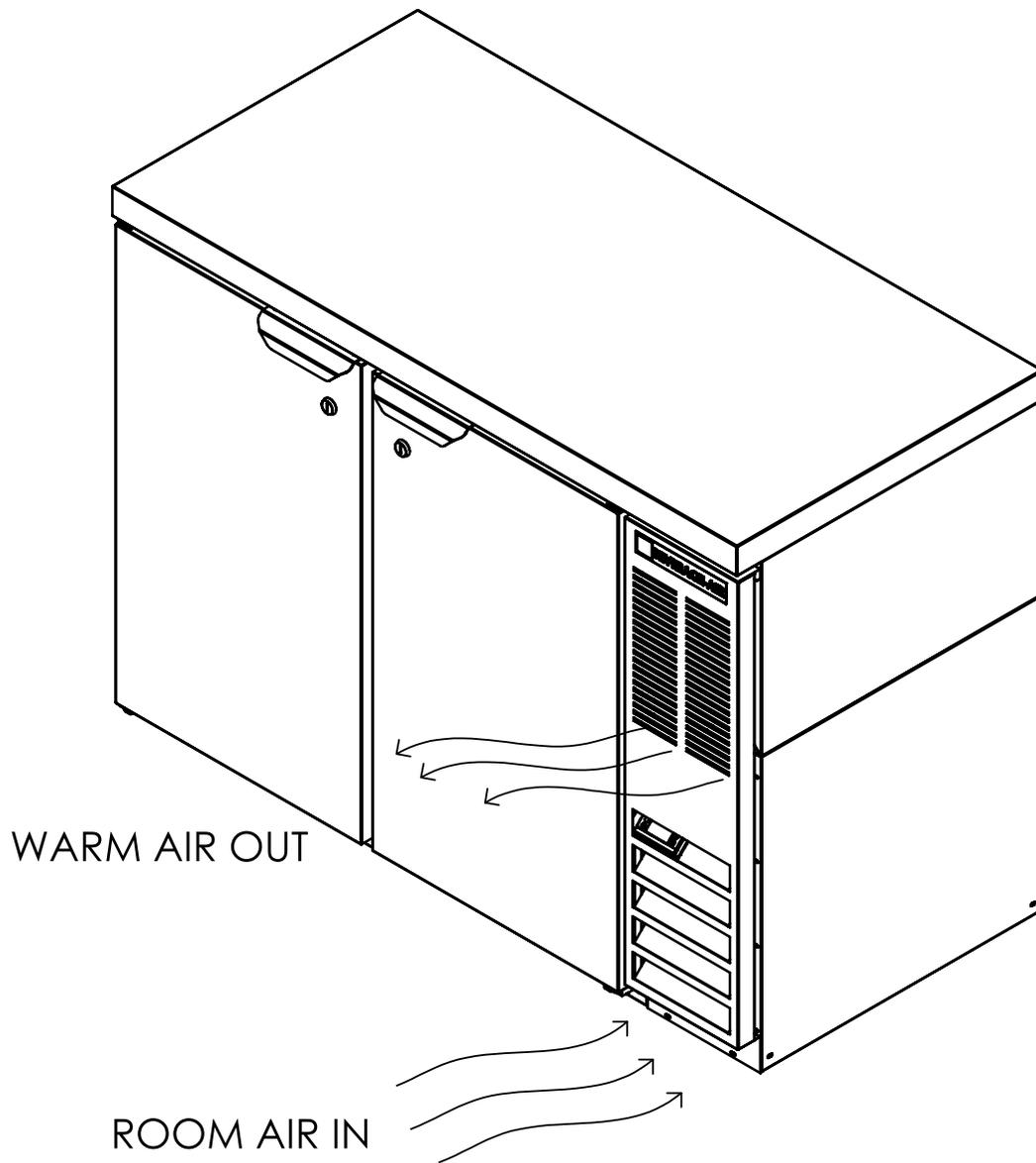
**Air Flow, 58 - 94 inch Models regardless of left or right grille location, section, door count or door material. Left grille shown, right grille similar but air flows in the right front, out the back and right side.**
