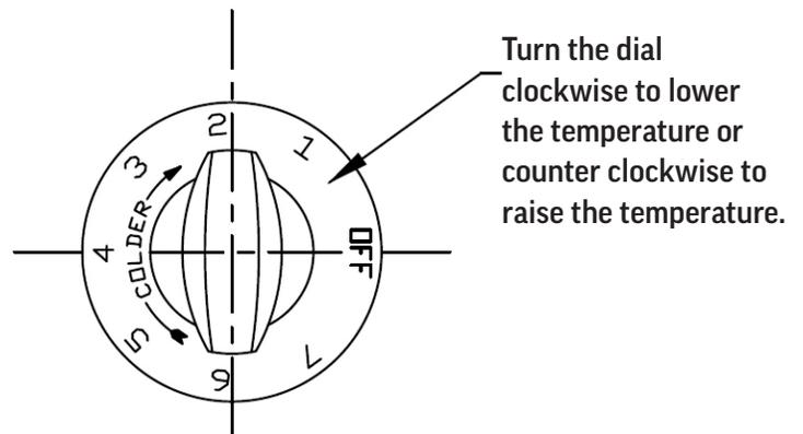
Excessive tampering with temperature control could lead to service difficulties.
