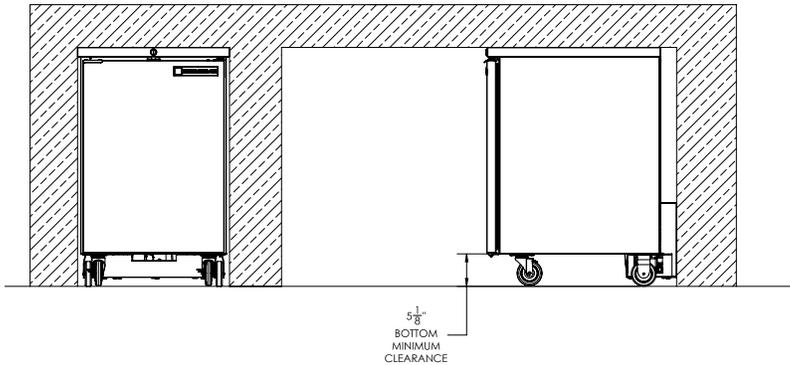
0 INCHES MINIMUM CLEARANCE AT TOP, BOTTOM, SIDES AND BACK.
