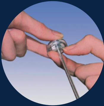
With Comark's patented calibration nut, you can easily calibrate your bi-metal thermometer in seconds with only a twist of your fingers. Once it is set, the nut stays tight and firmly in place. See [www.comarkusa.com](http://www.comarkusa.com) for further instructions.
