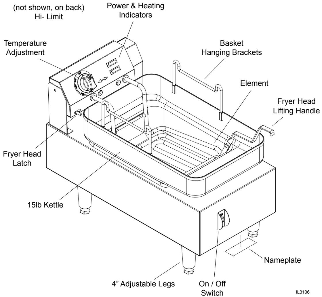
Fig. 1 Countertop Electric Fryer (shown with the fryer head in the down position)
