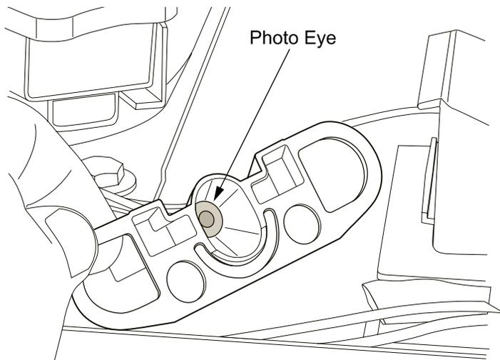
Note: Eye holders must be mounted properly. They snap into a centered position and are properly located when the wires are routed to the back and the left eye is the one with 2 wires at the connector.
