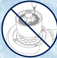
Sealed bearings eliminate the need to grease, while providing better reliability & lower service costs
