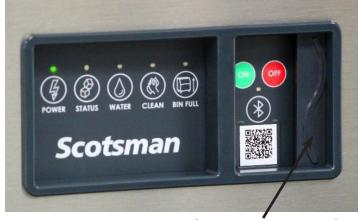
Open door to access On and Off switch buttons.
