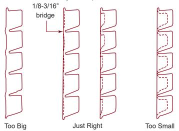
Bridge Thickness Adjustment Mechanism
