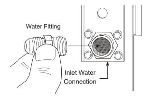
Water cooled models have a 1/2" FPT drain fitting plus an additional 3/8" FPT condenser inlet water connection.
