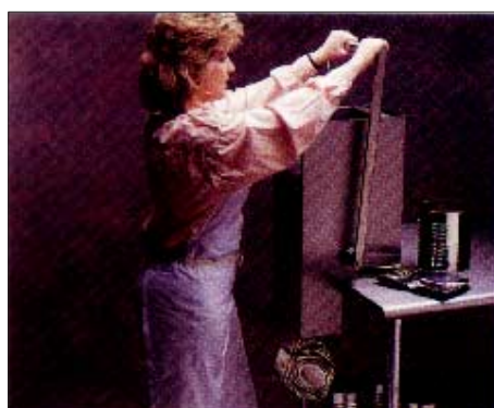
Return handle to upright position. Crushed can falls into receptacle.
