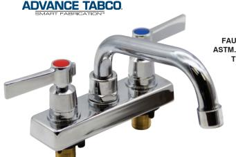
**FAUCET AERATOR CONFORM TO** ASTM.A112.18.1M • 1.0 GPM/3.8 LPM THREAD: 55/64 - 27 FEMALE
