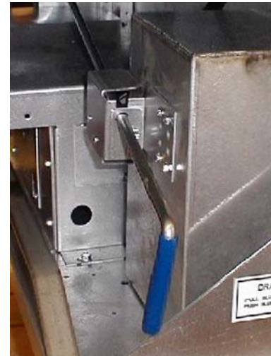
With the hose directed into the frypot, turn on the pump with the front-mounted switch.
