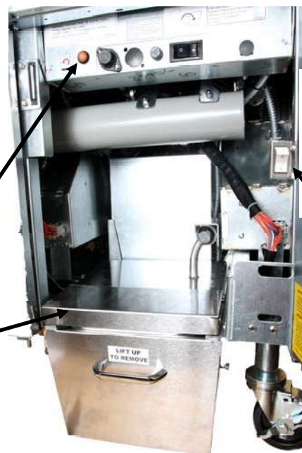
Figure 3: Plug the black connector into the utility box as shown. A separate harness with a white plug, if present, is NOT used.
