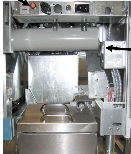
Melting unit power switch
