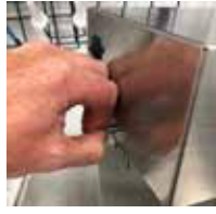
Pulling locking spring pin out to lock the back of the lid into position
