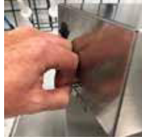
Pulling locking spring pin out to unlock the back of the lid
