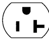
(1440 watt cabinets can be plugged into 20 Amp outlet)
